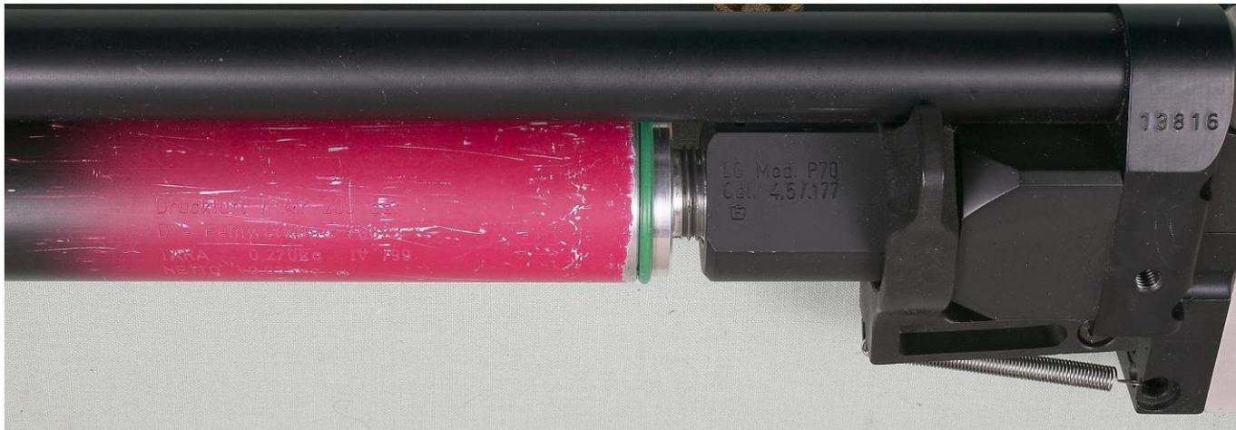
**Severe galling from misuse caused the cylinder on left to unscrew from the tube, allowing the cylinder body to become projectile.**
