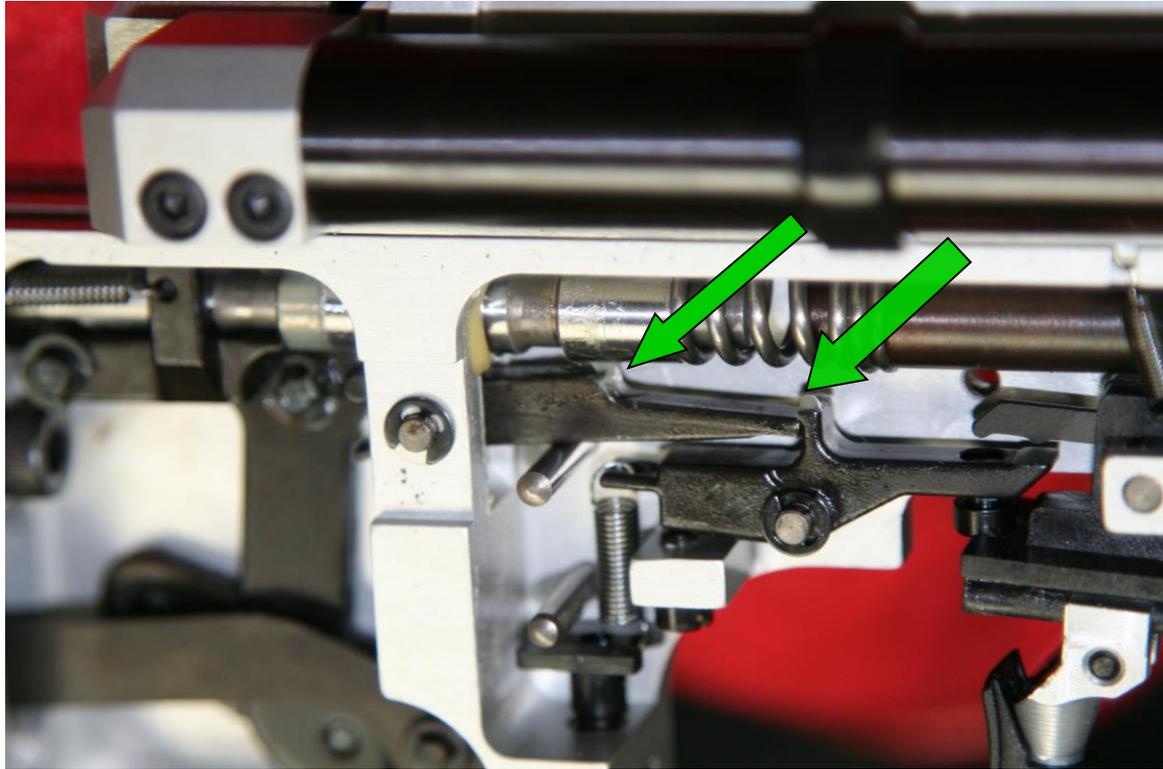
The high friction points of the sear and the valve catch link should have a very small amount of grease applied to their "bright" areas if they appear dry.
